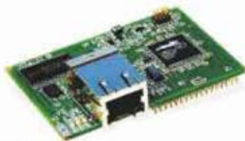
Fig. 2 Modulul RabbitCore 3200 (C-Programmable with Ethernet)
